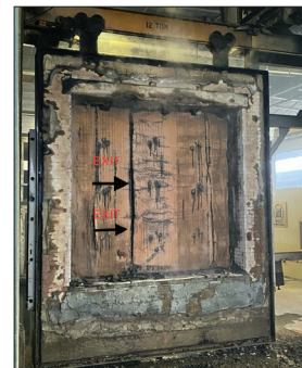
After Hose Stream Test First Responder Door Intact
