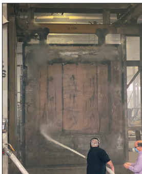
Hose Stream Application Does Not Open First Responder Door
