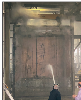
Hose Stream Application Does Not Open First Responder Door
