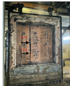
**After Hose-Stream Test First Responder Pass Through Slot Intact
