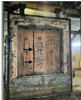
**After Hose-Stream Test
